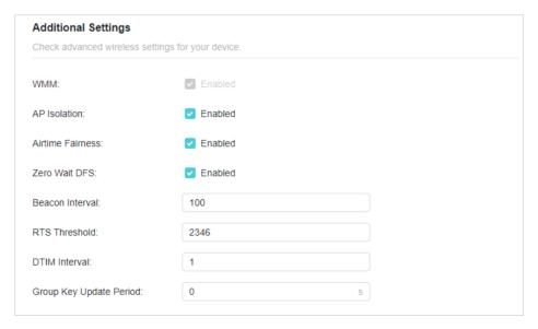
• WMM - WMM function can guarantee the packets with high-priority messages being transmitted preferentially. This function is enabled by default and uneditable.
