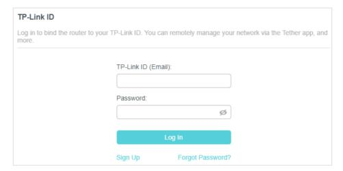
4. After activating your TP-Link ID, come back to the TP-Link ID page to log in. The TP-Link ID used to log in to the router for the first time will be automatically bound as an Admin.
