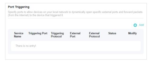
3. Click VIEW COMMON SERVICES, and select the desired application. The Triggering Port, Triggering Protocol and External Port will be automatically filled in. The following picture takes application MSN Gaming Zone as an example.
