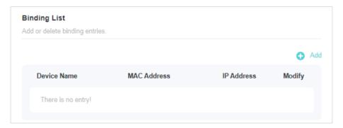
2) Click VIEW CONNECTED DEVICES and select the device you want to bind. The MAC Address and IP Address fields will be automatically filled in.
