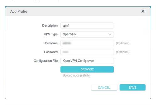
Note: You can also check the box of Import the CA file or edit the . ovpn file manually, then upload the CA file or manually configure the settings.
